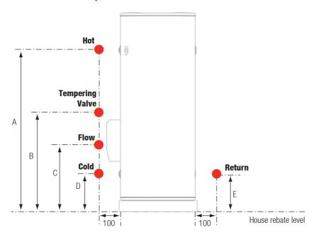
Approximate location of pipework. A tolerance of 25mm is acceptable to dimensions shown in table below. **Note:** Ensure pipes protrude horizontally from wall, and leave enough length of pipe to allow easy connections.
