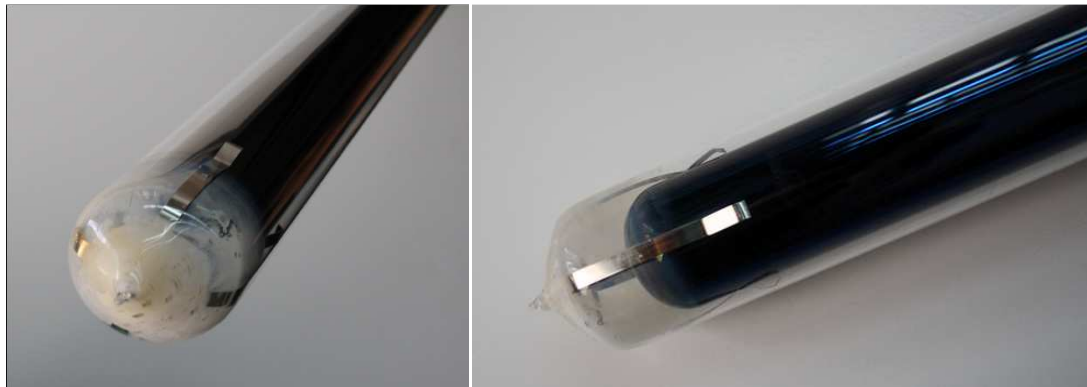
Tube with Loss of Evacuated Air
