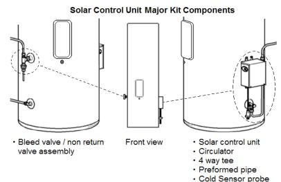
The solar control unit is mounted on the side of the solar storage cylinder and controls system operation. The solar control unit has a power cord which connects to a 240 volt general purpose outlet (refer to "Installation – Electrical & Electrical Connections" on page 28).
