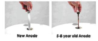
Solar Lord Enamel (glass) lined mains pressure hot water tank is fitted with a Sacrificial Anode, which protect the tank from corrosion. The Anode is "sacrificial", meaning that it is a softer alloy than the cylinder and all corrosion will occur at the Anode and not your cylinder. Sacrificial anodes do not last much longer than the standard warranty period of the tank.
