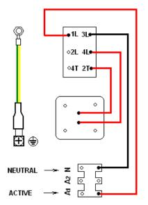
Electrical connections must be installed in accordance with AS3000 SAA wiring rules (in Australia) and local codes. All the electrical work must be undertaken by a qualified electrician. All solar hot water systems require a power outlet to run the pump. When using the gas booster an additional power outlet will be needed.
