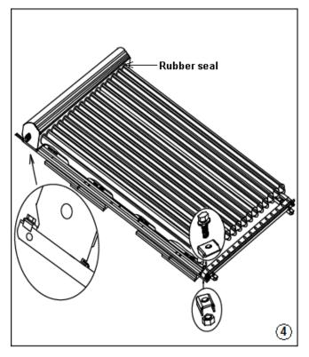
3) Replace tiles, then align stainless steel mounting tracks vertically and attach to roof mounting strips.
