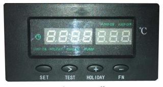
ler turns the circulating pump on or off according to the difference of temperature that has been preset. The pump is automatically turned on when the collector/s temperature is approximately **9**°C higher than the tank. It then is turned off when the temperature differential is **4**°C.
