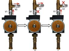
Step 1) Turn the ball valves to open position, fill the system with water until water steadily flows from the opened valve (V2).
