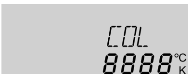
Channel indication upper line text display lower line temperature or temperature difference display
