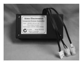
The System Controller is supplied with three sensor leads, one long and two short. Unroll each lead in turn and pass it through a small cable gland from the inside of the housing to the outside.
