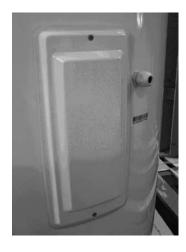
Step 1. Remove the housing cover by removing 2 screws.
