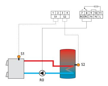
If the difference 1,6 K (hysterisis, can difference is reduced, cannot be changed) underruns the adjusted temperature difference, the pump is switched-off again.
