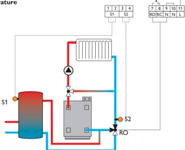
If the temperature difference  $\Delta T$  between store sensor S1 and heating circuit return sensor S2 exceeds the temperature difference adjusted at the controller, the 3-way-valve is switched-over. The return temperature of the heating circuit is raised by the heat of the store so that less conventional energy is necessary to reach the required flow temperature; in the course of this the temperature difference is reduced.
