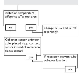
The temperature difference between store and collector increases enormously during operation; the collector circuit cannot dissipate the heat.
