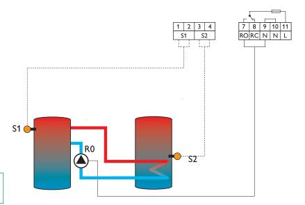
If the temperature difference  $\Delta T$  between store (1)- sensor S1 and store (2)- sensor S2 exceeds the temperature adjusted at the controller, the circulation pump is switched-on. Heat is transported from the store (1) into store (2); in the course of this the temperature difference is reduced.
