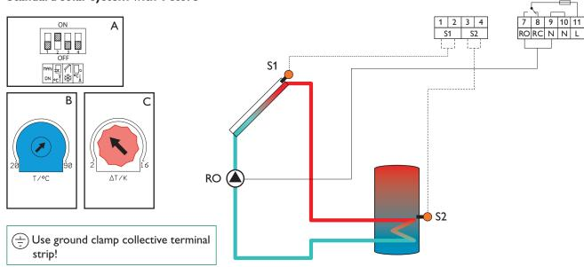
If the current temperature difference  $\Delta T$  between collector sensor S1 and store sensor S2 exceeds the temperature difference adjusted at the controller, the solar pump is switched-on. Heat is transported from the collector to the store; in the course of this the temperature difference is reduced. If the adjusted temperature difference is underrun by a difference of 1,6 K (hysteresis, cannot be changed), the pump is switched-off again.
