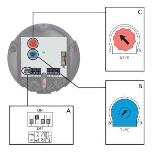
The micro-switch (A) activates (ON) deactivates (OFF) following functions:
