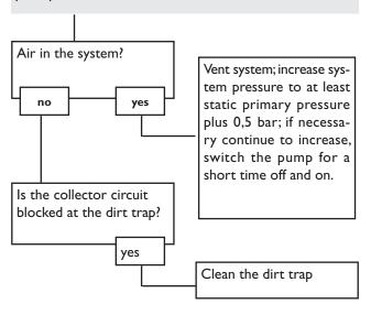
Pump starts for a short moment, switches-off, switches-on again, etc. (,,controller hunting")
