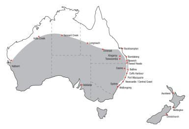
All locations highlighted in gray require an approved anti-frost protection device to maximise system performance. Call Dux Hot Water 1300 365 115 for further information.
