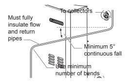
Ensure flow and return pipes from the solar collectors to the water storage tank have a minimum of 5° continuous fall
