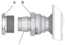
Ensure the brass conetite compression fitting is installed in the correct direction
